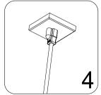
slide the eyehole bracket into endcap to secure the fixture in place as shown above. Repeat these steps on the other side of the fixture. Confirm that the screws are tightened
