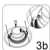
3b. Before installation For 5 in. recessed housings: Slide the torsion spring bracket to 5 and tighten screw using a Phillips head screwdriver. For 6 in recessed housings: Slide the torsion spring bracket to 6 and tighten screw using a Phillips head screwdriver. Note: Applicable to LED25DRS6UB/G4/CCT9Q.
