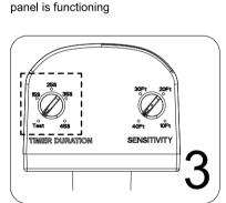
Set up motion sensor timer (knob is located on the bottom of motion sensor head). This sets the amount of time the light stays on at 100% brightness after motion is detected. Select from these durations: 15/25/35/45
