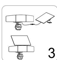
The solar panel must receive direct sunlight over 5 hours per day to keep the battery charged. If your fixture is mounted on a north/east/west facing wall or obstructed from sunlight, mount the solar panel remotely (4A). If your fixture placement receives ample sunlight, then mount the solar panel onto the fixture (4B).
