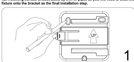
the bracket away from the fixture. Place the mounting bracket flush to the wall with the arrow on the bracket pointing UP leaving at least 4-inches of flat surface to the right of the bracket location. Mark the three hole locations. Put the panel aside and drill three pilot holes using 7/32" drill bit. Note that all steps are the same for all models.
