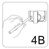
Remote solar panel installation. a south facing location exposed to sunlight (must be within 118" from the light panel). Hold the solar panel in place and mark both hole locations on the mounting surface. Put the solar panel aside and use a 7/32" drill bit to create two pilot holes. Insert plastic anchors same as in step 2. Align the holes of the solar panel mounting bracket to the plastic anchors and use the screws to secure the solar panel to the mounting surface.
