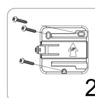
plastic anchors into the pilot holes. Ensure that the anchors are tapped all the way in. Align the bracket over the holes and insert screws. Tighten screws with a Phillips head screwdriver.
