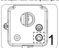
Press the On/Off button to confirm the fixture lights up. It will light up for about 15 seconds when powered on for the first time and will light up for about 4 seconds when the color temperature button is pressed. **NOTE:** This fixture contains a rechargeable battery. If the fixture does not turn on, please connect the solar panel and charge it for a few hours under sunlight. Then press the On/Off button to confirm that the light
