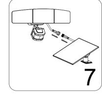
Connect the wire between solar panel Press the On/Off button to turn on the fixture. Note that the fixture will turn on for 4 seconds and will turn off if daylight is sensed.
