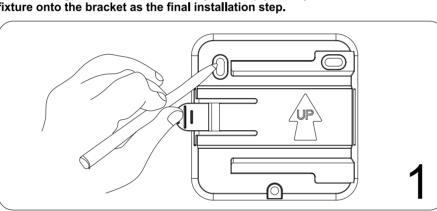
Remove mounting bracket from the back of the fixture by pressing the tab and pulling
