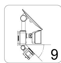
Tilt the motion sensor head to detect motion closer or further from the fixture location. Note: The side of the knob is facing downwards.
