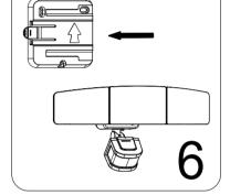
Slide the fixture into the mounting bracket from right to left.
