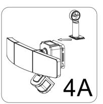
On-fixture solar panel installation. The fixture and solar panel should be mounted in a south facing location exposed to sunlight. Slide the solar panel bracket onto the top of the
