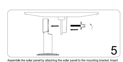
the thumbscrew into the hole and loosely tighten. Adjust the vertical tilt to 25-45 degrees and then tighten the thumbscrew. Note: this step is the same with or without the solar panel attached to the fixture.
