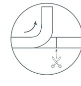
With your Light Strip unplugged, safely cut where the trim points are indicated. ▲ Make sure the strip is not plugged
