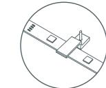
Lay out mounting clips where desired.
