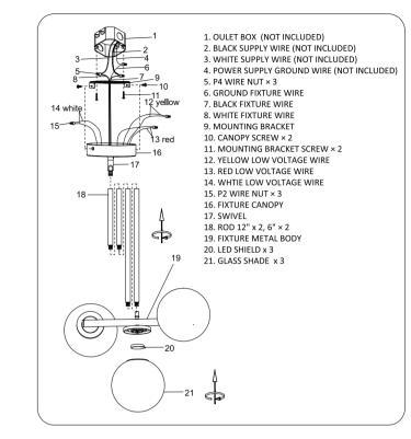
6. Connect black supply wire[2] to black fixture wire[7] and connect white supply wire[3] to white fixture wire[8] by using P4 wire nuts[5]. Connect ground fixture wire[6] at the top of the fixture canopy[16] to power supply ground wire[4] from outlet box[1]. Wrap P4 wire nuts[5] with electrical tape for a more secure connection. Carefully tuck wires back into the outlet box[1]. Do not get wires pinched between ceiling and canopy.
