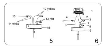
Attach fixture canopy[16] onto mounting bracket[9] using canopy screws[10]
