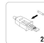
Remove fuse carefully. Risk of fire. Replace fuse only with 5 Amp, 125 Volt fuse. Failure to do so may be a fire hazard. 1pcs fuse contained in the plug.
