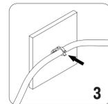
You may use the included mounting clips to secure the Rope Light. Fix Mounting Clips with Screws onto surfaces and snap Rope Light into place.
