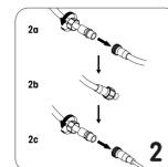
You may link additional sets of Rope Lights (up to 200 ft) by unscrewing the plastic cap at the end of the Rope Light to access connection port(2a). Leave it covered if you do not want to link additional lights(2b). Connect the Rope Light to the Power Card by screwing the plastic end cap tightly to the Rope Light(2c).
