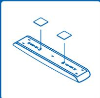
Attach the double-sided tape to the back cover of light bar, then stick the bar to a dry and clean location.
