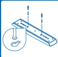
Install two screws to mounting surface with 4.3 inch gap, as shown above. Hang light bar to the screws.
