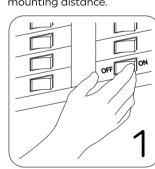
Turn off power source to the power supply where you are installing the fixture.
